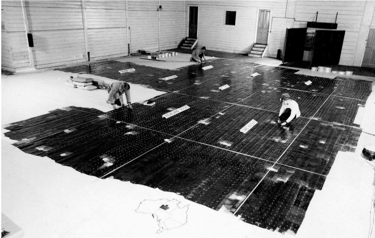
Figure 8 – Example of a large template assembly (8,300 templates approximately) covering an area about that of Victoria (courtesy P. Hocking).
