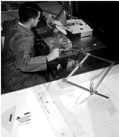
Figure 9 – Plotting from aerial photography using a Stereotop (Zeiss) and Radial Line Plotter (Kail) (courtesy D. Young).
