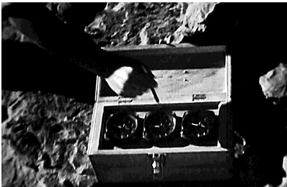
Figure 7 – Aircraft type barometer set (courtesy P. Hocking).
